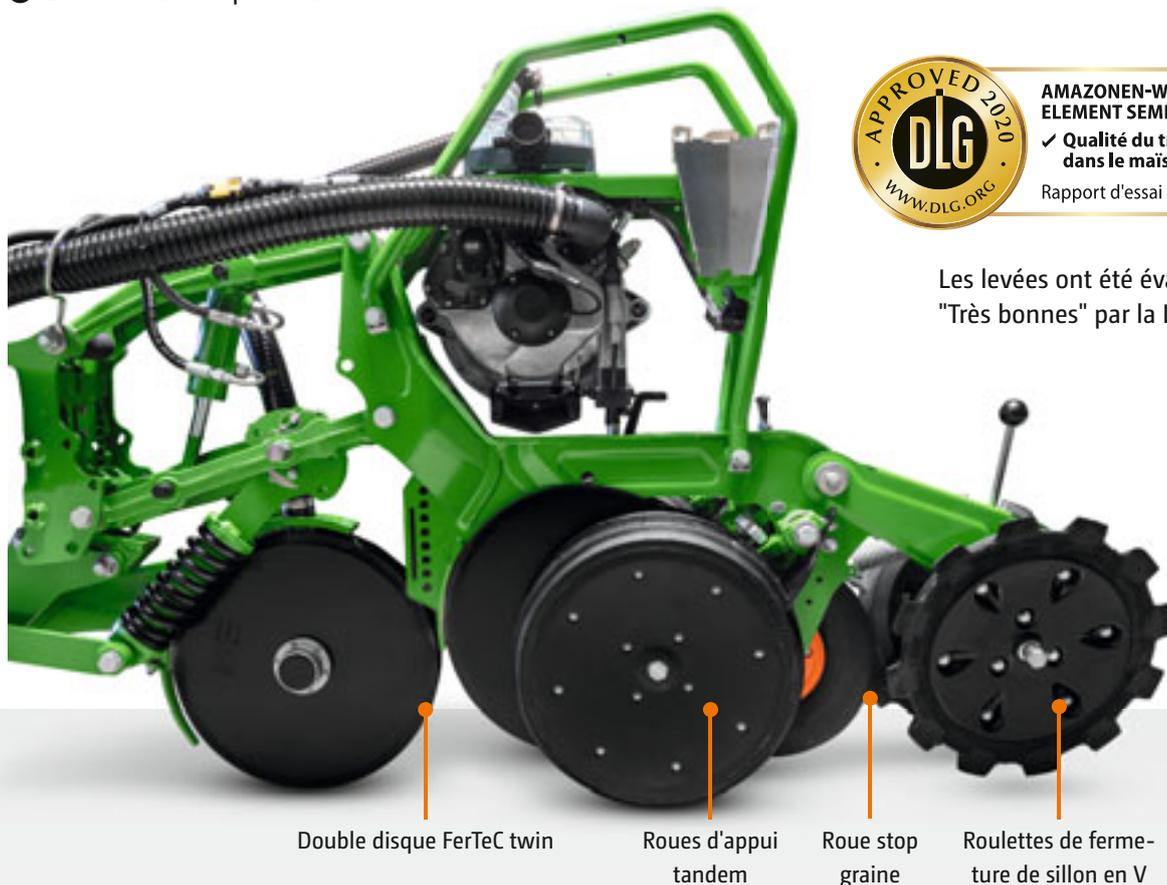
Double disque FerTeC twin
