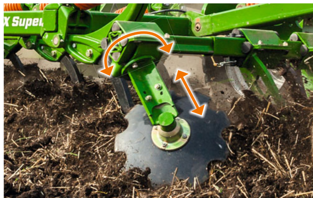
The outer closers – individually adjustable in height and angle
