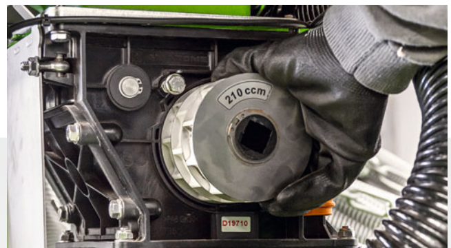
Easy exchange of the metering rollers
