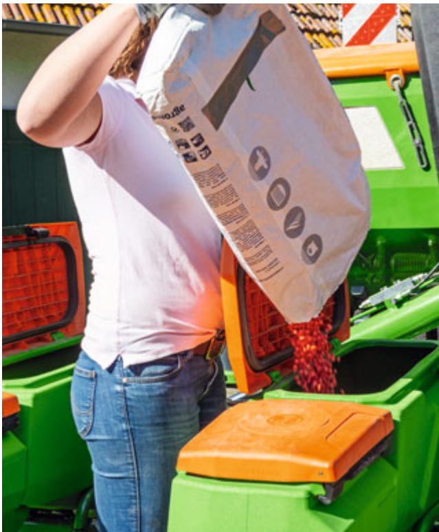
The seed hoppers are easily accessible and facilitate one-handed operation for opening and closing.
