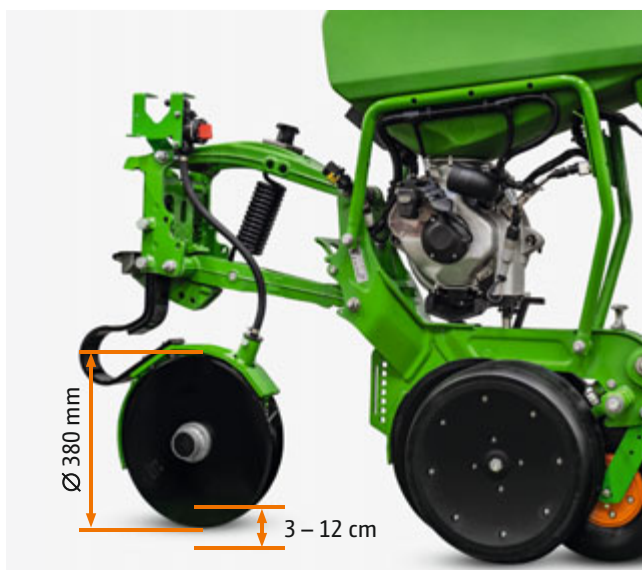
FerTeC twin fertiliser couler with leaf spring overload protection The placement depth is adjustable between 3 – 12 cm, and the maximum couler pressure is 80 kg
