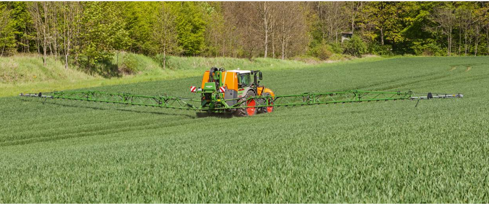
The UF 2002 mounted sprayer with ContourControl for fully automatic boom guidance
