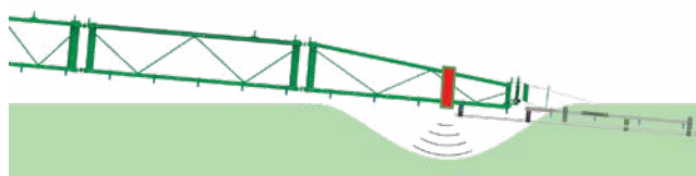
DistanceControl when equipped with two sensors: the boom can dip into the crop, for example, where there is lodged corn
