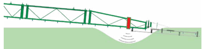
DistanceControl when equipped with two sensors: the boom can dip into the crop, for example, where there is lodged corn
