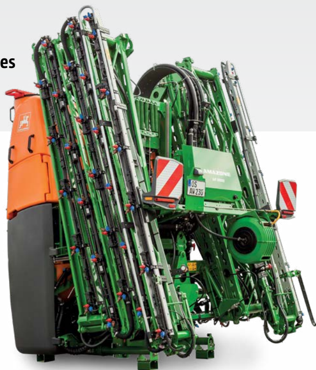
UF 2002 with Super-S2 boom in a 30 m width
