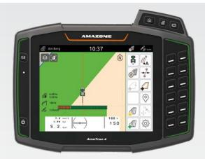
Overlaps on the headland or in wedge shaped fields are prevented via precise switch points with GPS-Switch.
