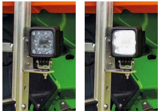
The pre-set weight is reached when the work lights come on continuously.
