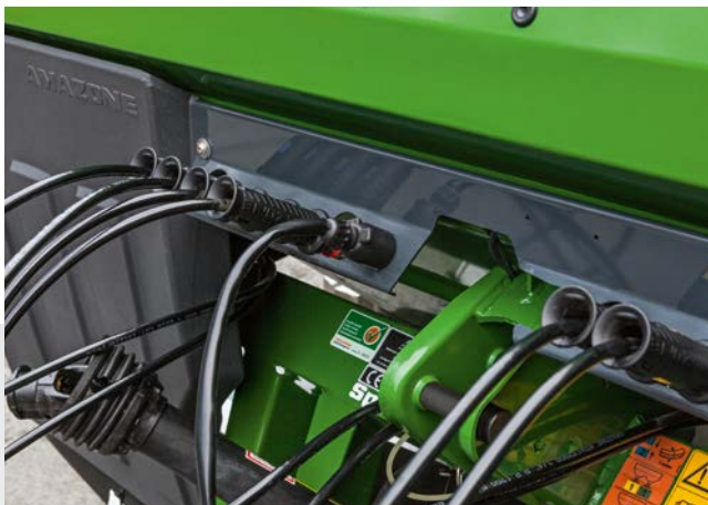
Accessible holder for the hydraulic hoses
