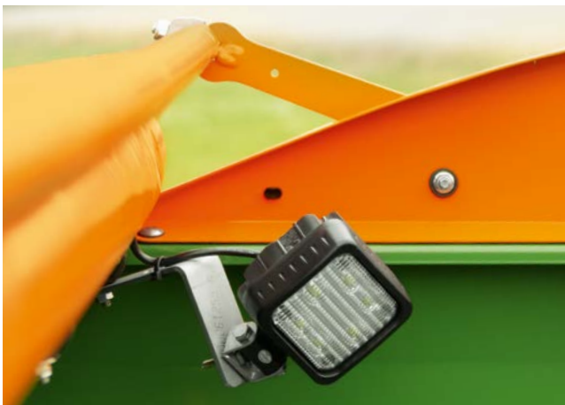
Internal hopper lighting
