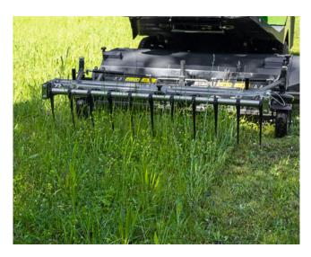
The InsectGuard tine carrier agitates the grass vigorously before the mower passes over it, scaring away insects. Protect nature with InsectGuard for Profihopper 1250 and 1500!
