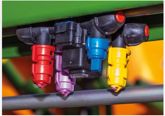
✔ AmaSelect electric individual nozzle control
