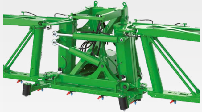
Swing compensation system for Super-L3 booms from 39 metres
