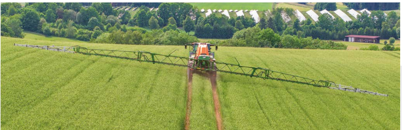
Low risk of tipping over in hilly terrain thanks to automatic slope compensation
