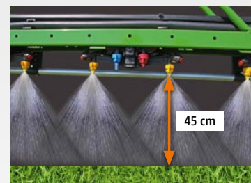
80° nozzles: 25 cm nozzle spacing
