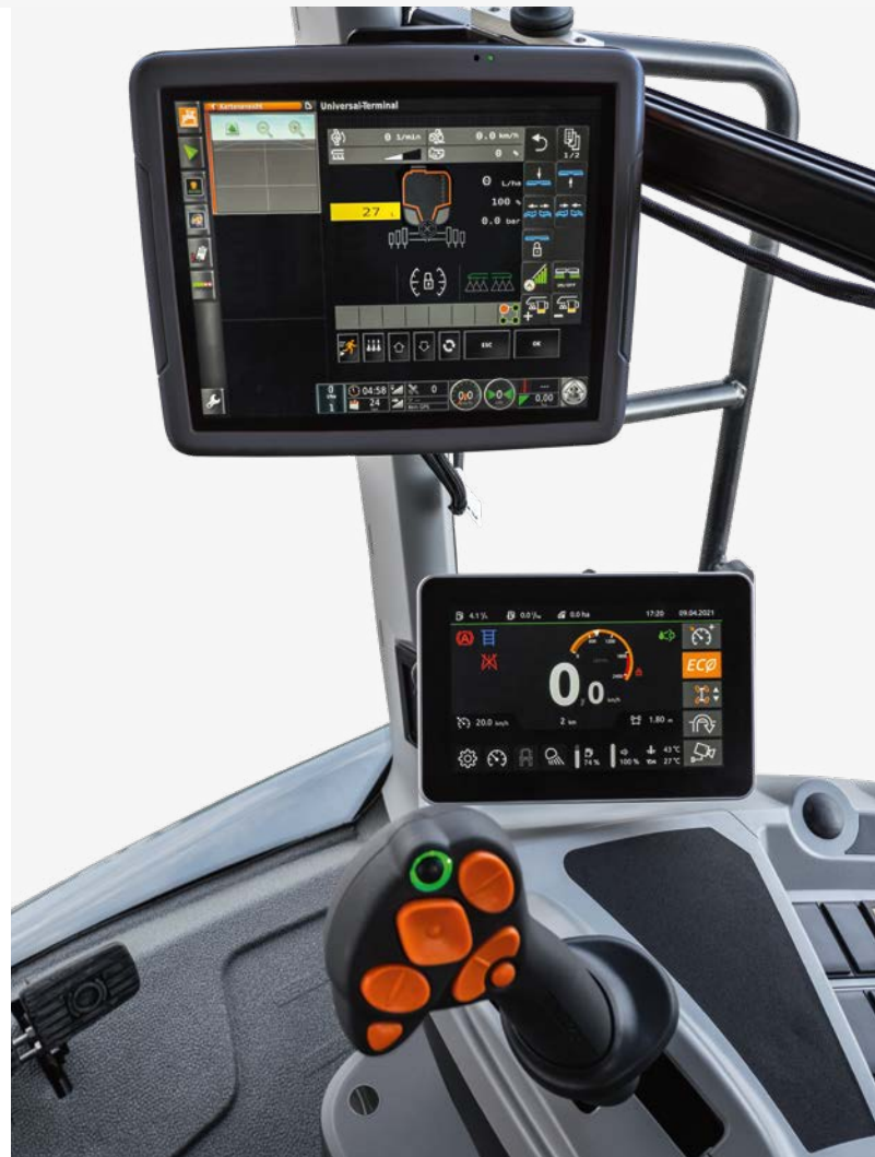
Twin-terminal solution with the TopCon X35 ISOBUS terminal and AmaDrive 7.0 vehicle terminal as well as the AmaPilot + multi-function joystick
