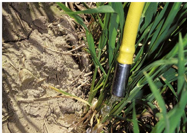
Stainless steel weights on the drag hose
