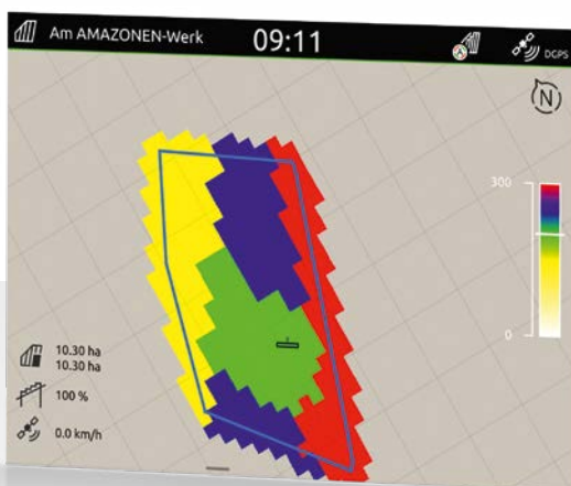
Display of the application map in AmaTron 4
