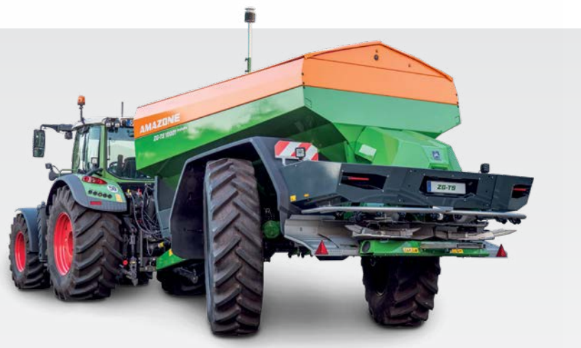
Steering axle with a steering angle up to 28°
