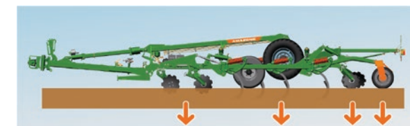
Ceus-2TX with all soil-engaging elements in the operational position
