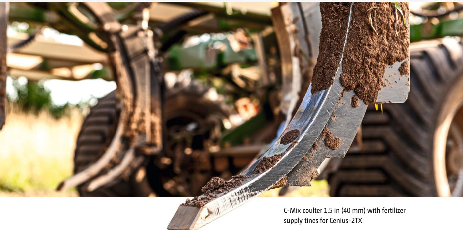
C-Mix coulter 1.5 in (40 mm) with fertilizer supply tines for Cenius-2TX
