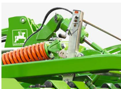
Spindles for central adjustment of the leveling unit on the Cenius-2TX
