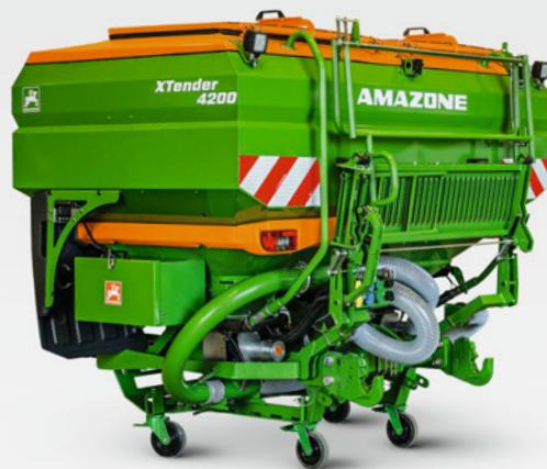
XTender 4200 mounted hopper with a capacity of 148 cu ft 120 bu (4,200 l)
