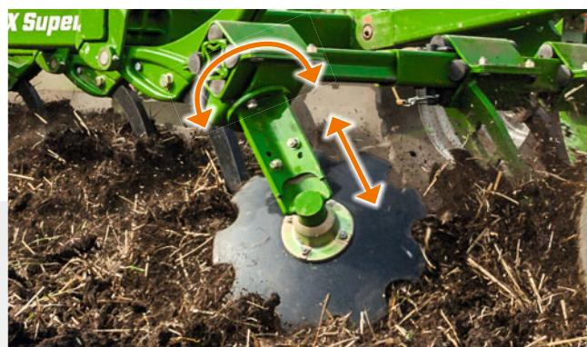
The outer closers – individually adjustable in height, angle, and position
