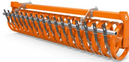
Spring-mounted clearing system for UW rear rollers
