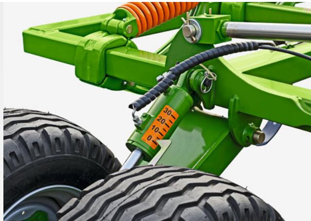
Setting scale for the fully hydraulic depth adjustment of the tine
