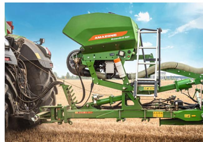
GreenDrill 501: for all trailedd machines – with a 14.2 bu (500 l) hopper and hydraulic blower fan
