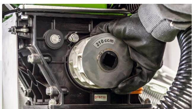
Easy exchange of the metering rollers
