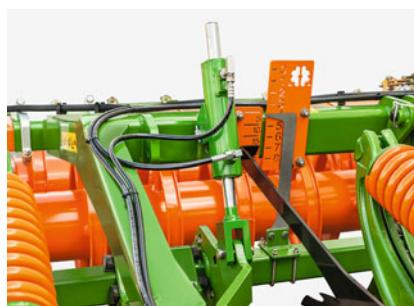
Hydraulic cylinder to set the depth of the leveling unit
