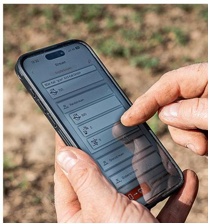
The settings can be sent to the machine from a smartphone via a Bluetooth connection.
