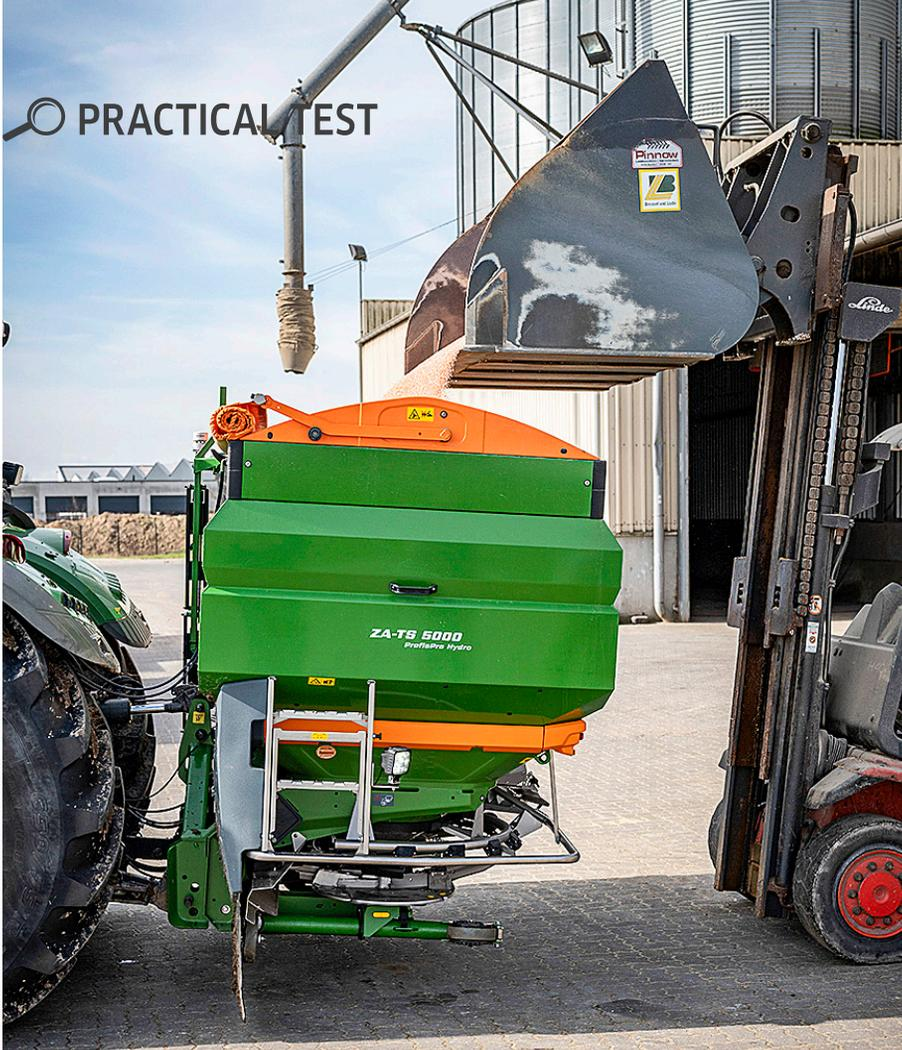
The cover opens wide and clear. The working lights help with filling – blinking as you approach the machine's maximum weight and staying on once you have reached it.
