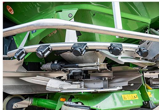
The ArgusTwin radar sensors reliably monitor the machine's spreading pattern.
