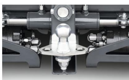
Trailer coupling, complete with strapping points<sup>2+3</sup>
