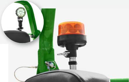
LED work lights and/or flashing beacon
