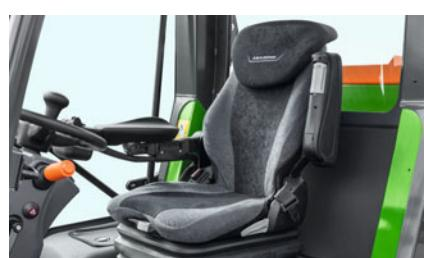
Various seat options, such as the Grammer "De Luxe" seat with air suspension and heating
