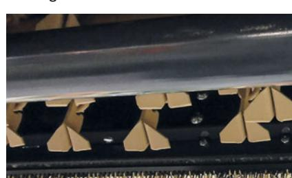
Polyurethane-coated support rollers
