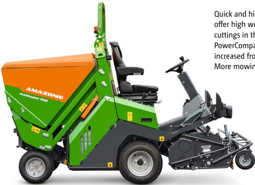
Quick and highly-manoeuvrable - the Profihopper 1250 offer high work rates and maximum consolidation of the cuttings in the collection hopper thanks to the PowerCompactor - the effective capacity of the hopper is increased from 730 l to up 1,000 l of collected cuttings. More mowing, less downtime.
