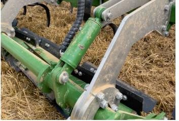
The intensity of work of the knife roller is controlled hydraulically so operators can raise it out of work conveniently.
