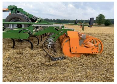
The parallelogram frame ensure consistent ground contact. Excellent.
