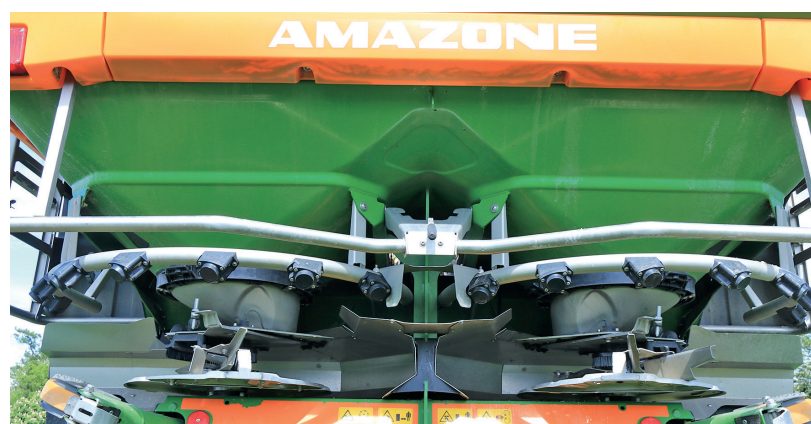
A total of 14 radar sensors (the black components on the pipe hanger) monitor the discharge angle of the spreader.
