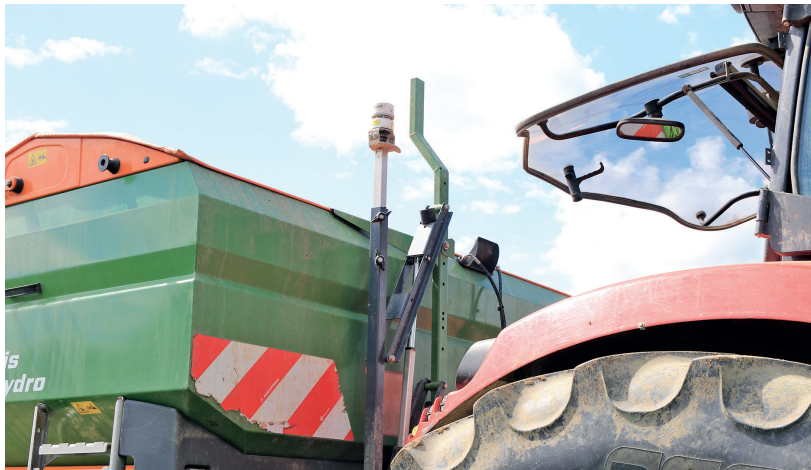
When folded into the transport position, the wind sensor remains within the height of the vehicle.
