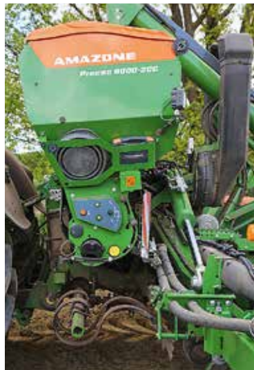
This fertiliser hopper has a capacity of 1,250 litres. Access to all calibration points is good.
