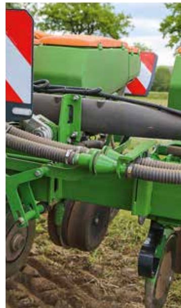
The outer fertiliser delivery tubes couple/uncouple automatically during folding.
