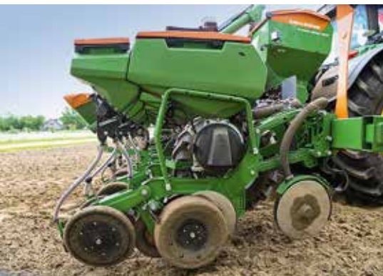
The seed tanks hold 70 litres now. The photo shows the unit with fixed and adjustable fertiliser couler.
