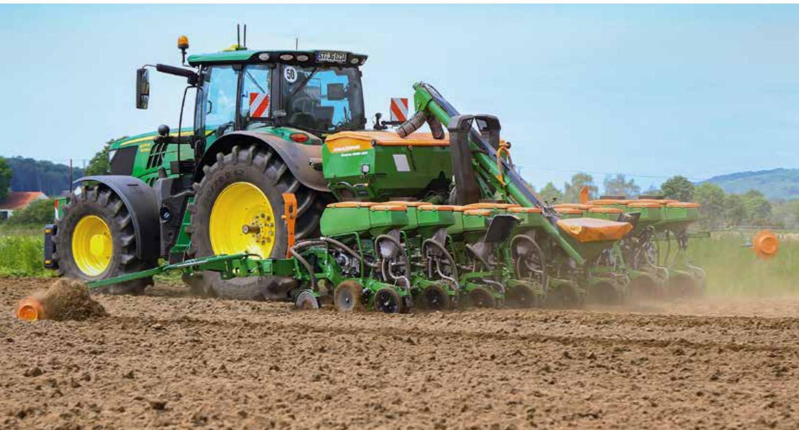
We put a 6m Precea prototype through its paces planting eight rows of maize spaced 75cm in one pass. Photos: Schulz, manufacturer (2)
