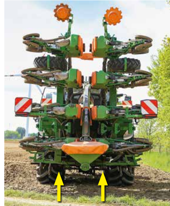
Note that the frame sections on either side of the filling auger have different lengths.
