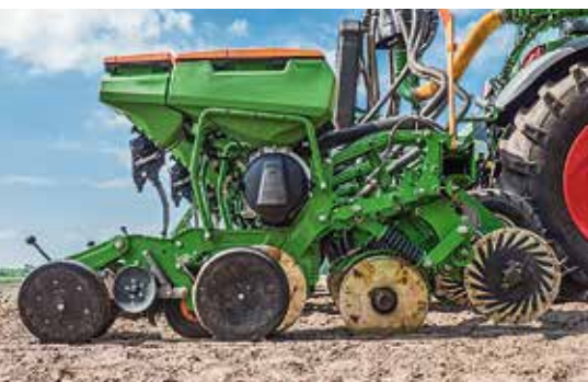
A fertiliser couler is available as an option. This maintains its placement depth relative to the seed depth.
