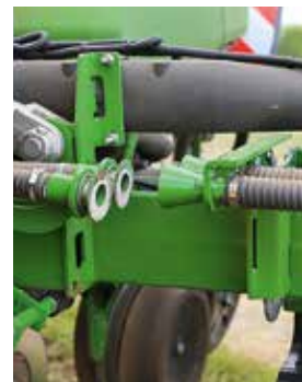
The outer fertiliser delivery tubes couple/uncouple automatically during folding.
