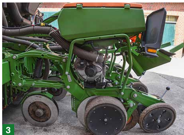
△ 1) Fertiliser calibration testing is done on the left machine side. 2) The singling discs are swapped without tools. 3) The pressure on the coulters is applied by springs.
