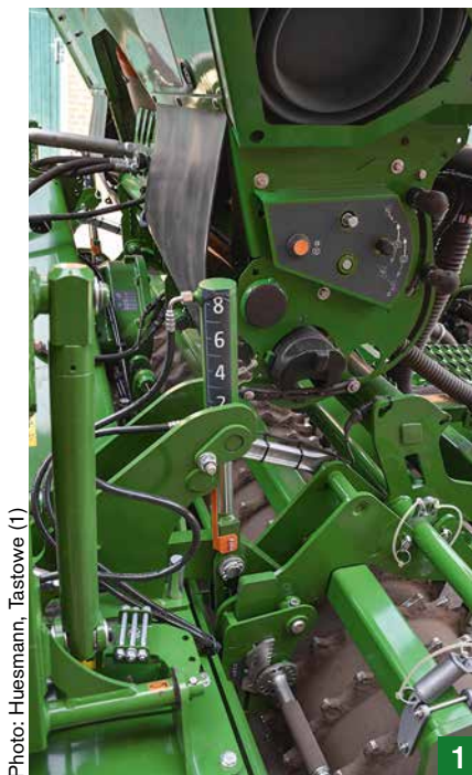
△ 1) Fertiliser calibration testing is done on the left machine side. 2) The singling discs are swapped without tools. 3) The pressure on the coulters is applied by springs.
