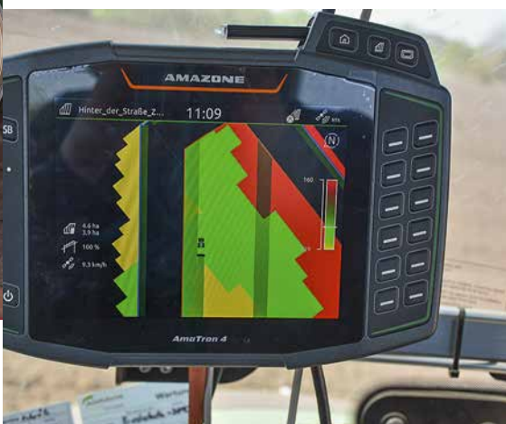
△ The fertiliser and seeds were applied using application maps from the Amatron.
