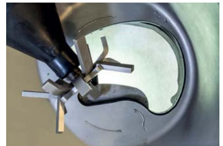
Stage 3: hopper aperture wide open
