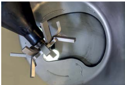
Stage 1: hopper aperture slightly open
