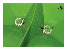
A twin hopper; that means automatic monitoring. If one side empties quicker than the other it can immediately be checked whether something is blocking the opening or whether the levers are evenly positioned on the stops. The twin hopper design gives optimized steep hopper walls, which guarantee – unlike single tip hoppers – a very constant fertilizer flow, even on slopes or with very little fertilizer left.
