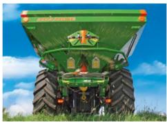
The twin disc spreader is for smaller to medium sized arable farms and grassland farms. The ZA-X Perfect allows convenient adjustment and the accurate spreading of all commercial types of fertilizer up to 60 ft (18 m) and with Urea up to 50 ft (15 m).
