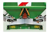
For fruit and hop gardens, the fertilizer is distributed around the plants by the easily adjustable twin-row spreading device, which leads to considerable savings in fertilizer application between the rows. Row spacing is from 6.5 ft to 20 ft (2 - 6 m).
