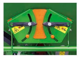
The spread rate adjustment with its two individual setting shutter slides is located well out of the "dirt range" meaning that they are neither splashed from the tractor wheels or with fertilizer dust from the spreading discs. In this way the machine remains clean and easy to operate. The pointers are arranged on a large, clear scale so that different rate settings such as border spreading are immediately obvious.
