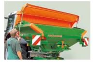
When filling, the swivel hopper cover (special option) is simply folded open and ensures dry material even when spreading in wet weather. A traffic light kit with warning plates (special option) is available upon request.
