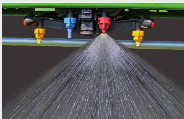
AmaSelect electric individual nozzle control with 4-fold nozzle body and 50 cm or 25 m nozzle spacing
