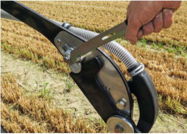
Setting the depth-guided tine coulters
