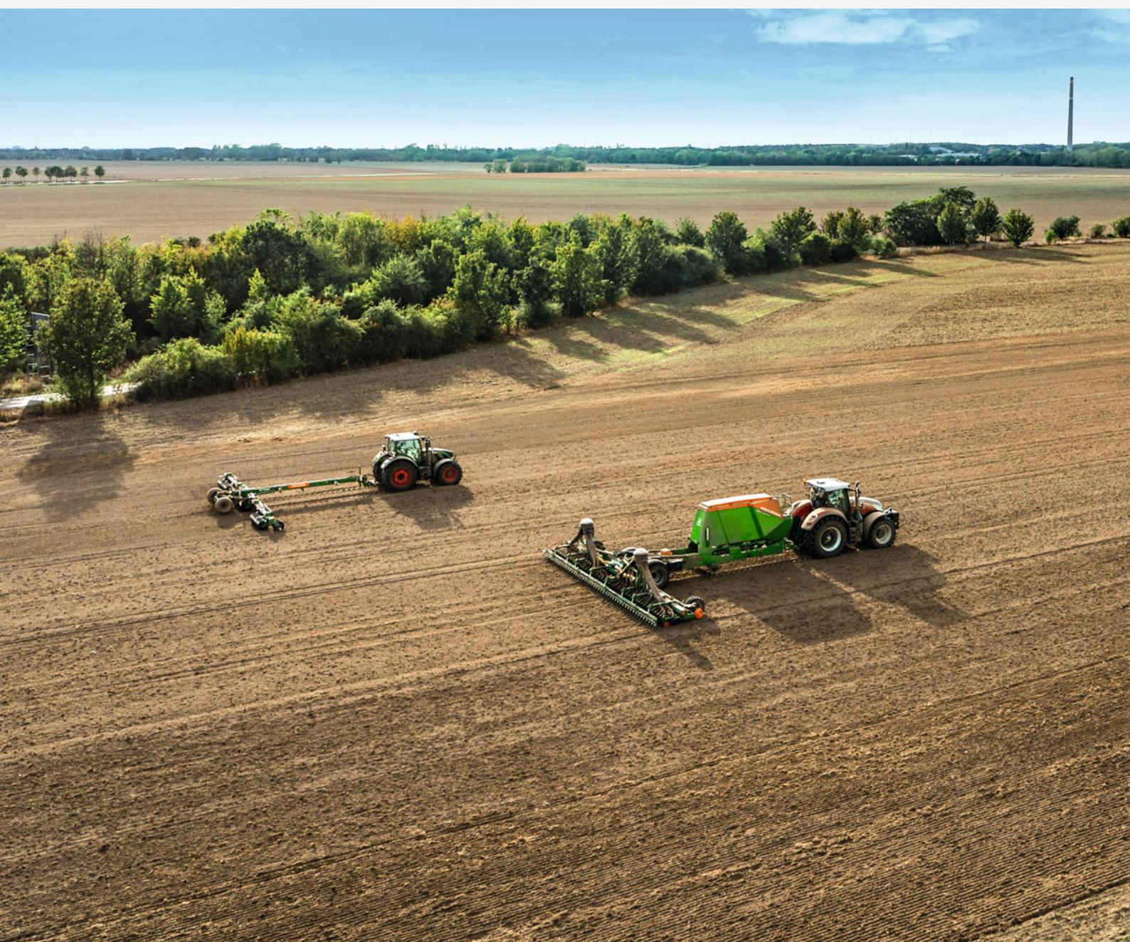
Due to its easy pulling and working widths of 12 m and 15 m, the Citan trailed seed drill easily gets over the acres. With its 7,800 l hopper capacity, the Citan provides farmers with enormous efficiency, particularly for use on large farms with short sowing time frames. The Citan is equipped with a 3-section pressurised tank as standard, which can also be used to place fertiliser in the seed furrow.
