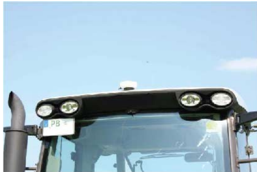
GPS receiver on the roof of a tractor
