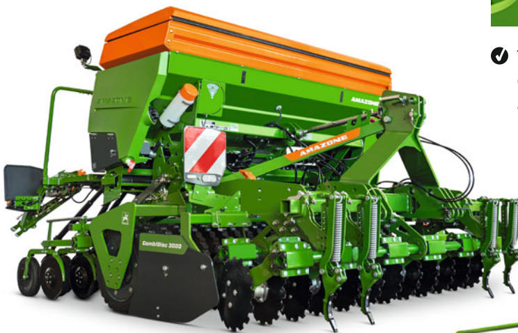
CombiDisc mounted compact disc harrow with harrow-mounted Cataya 3000 Super seed drill
