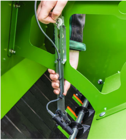
The simplest of conversion from fine to normal seeds using the shutter slides
