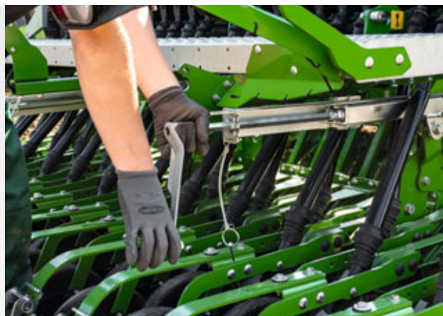
Simple setting of the placement depth, from the right and left, at the back of the Cataya Special
