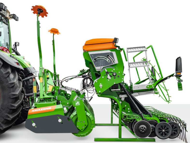
Cataya Special with TwinTeC special double disc coulters
