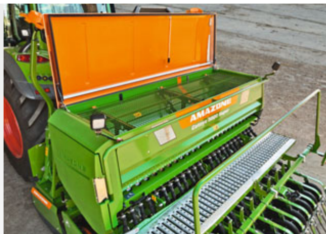
Sieves in the hopper protect the operator
