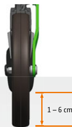
Working depth of the Control 50 depth guidance roller
