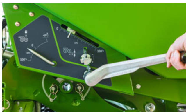
Central, infinitely-variable mechanical coulter pressure adjustment with setting scale on Cataya Super
