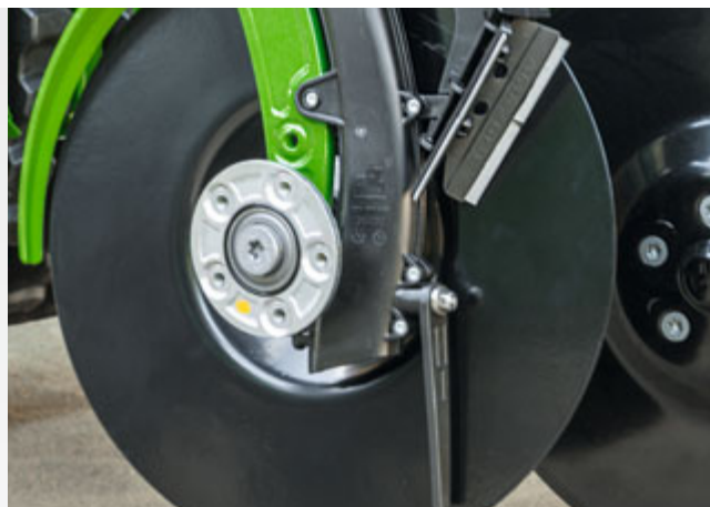
The hard metal internal scraper for sticky clay soils ensures problem-free coulters travel
