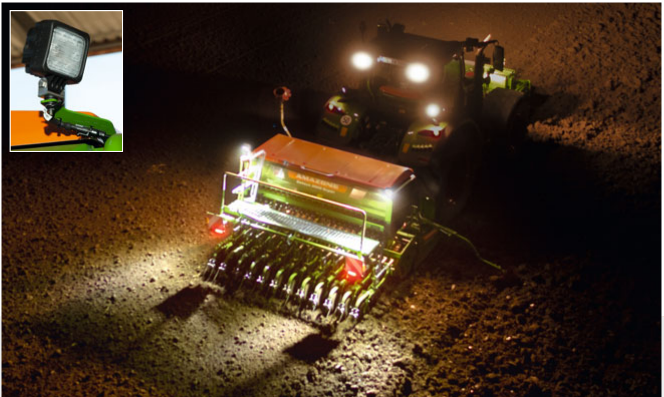
Improved vision at night via the optional LED working lights
