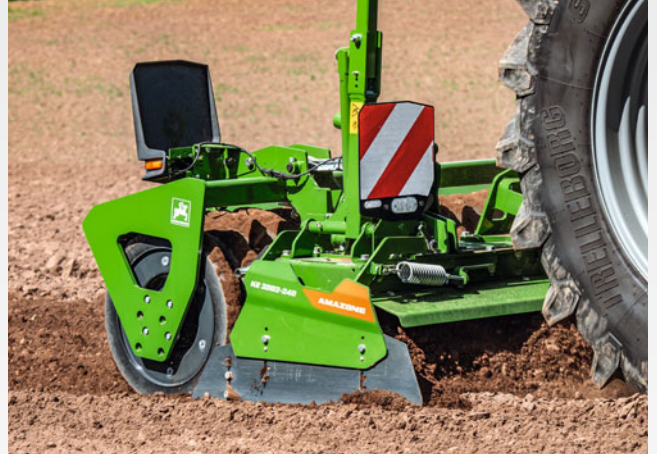
KE 3002-240 Rotamix rotary harrow in solo use
