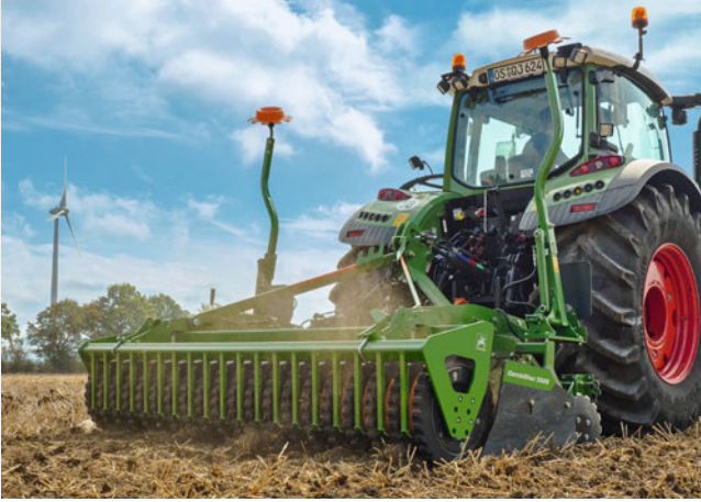
CombiDisc 3000 mounted compact disc harrow in solo operation
