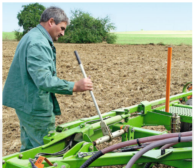
Basic setting of the sowing depth
