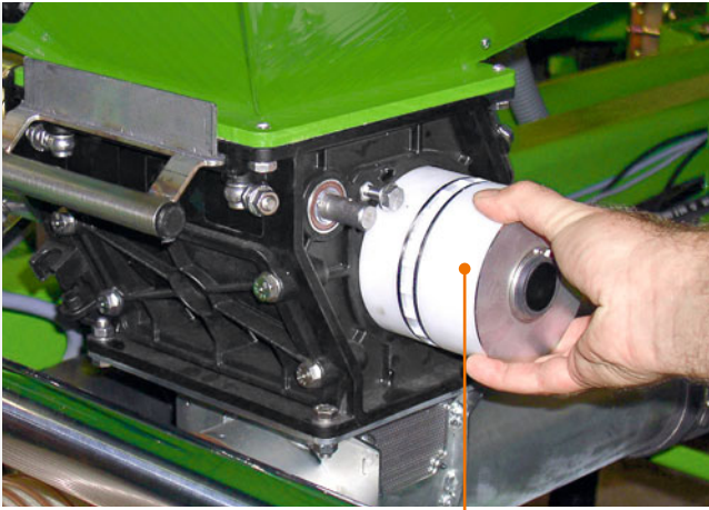
The metering cassettes, located to the front left hand side of the machine are quickly exchanged
