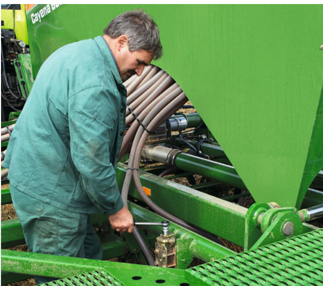
Basic setting of the Exact harrow S
