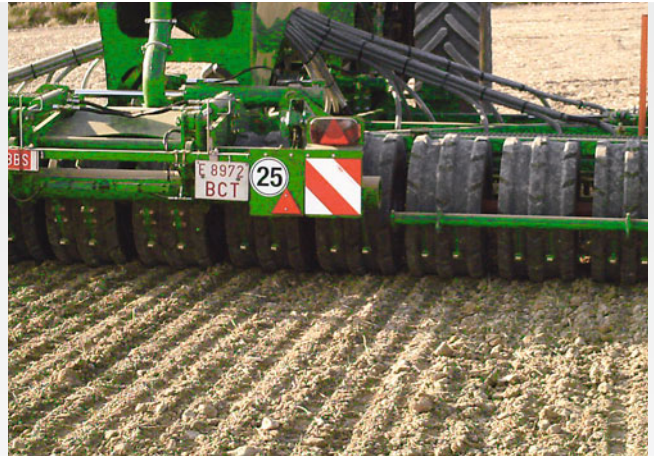
Wedge ring roller with matrix tyre profile
