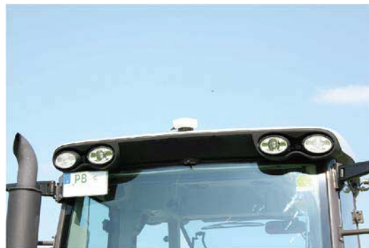
DGPS receiver on the roof of a tractor
