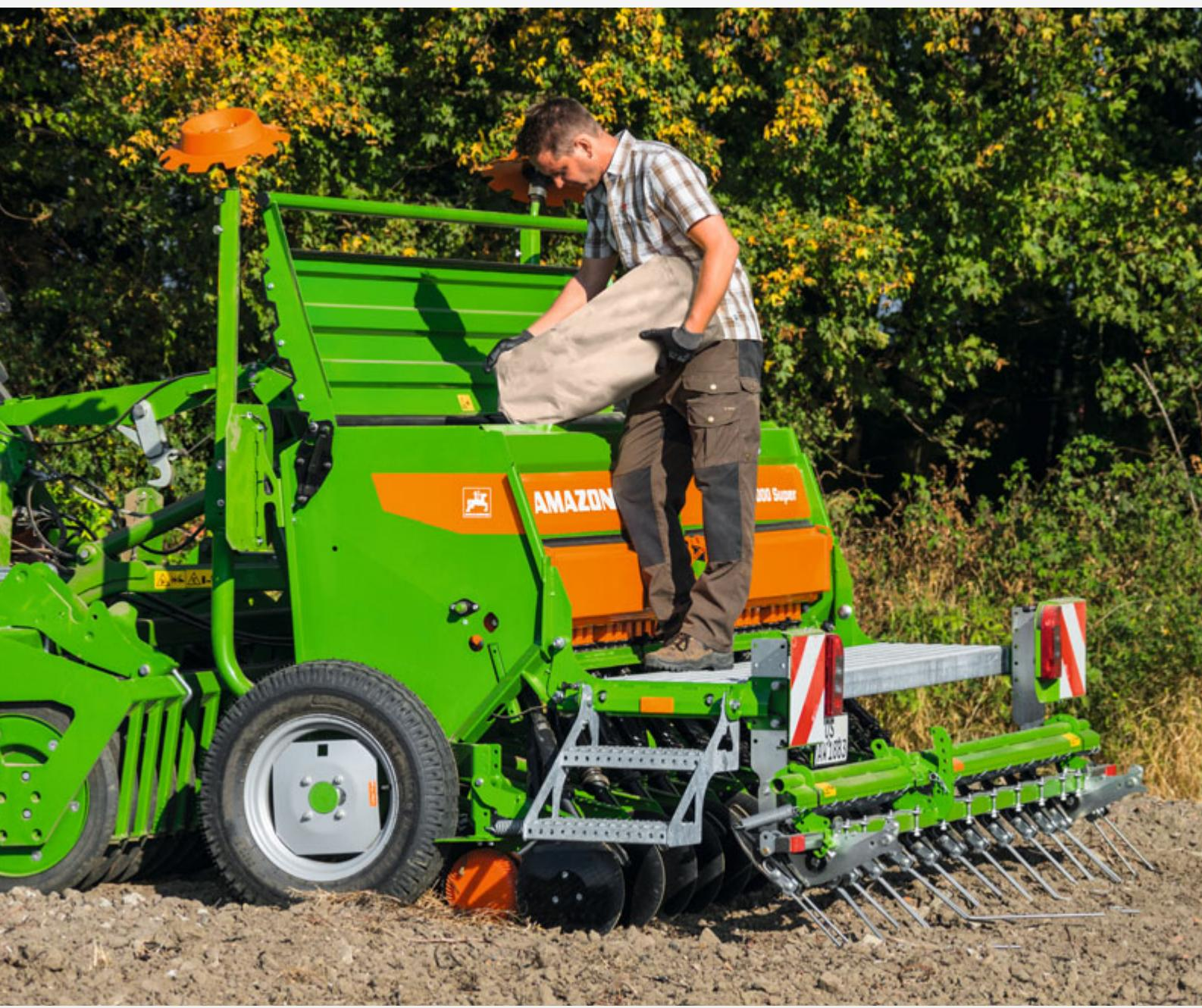
The safe access via the folding steps and the loading platform provides easy access to the seed hopper.
