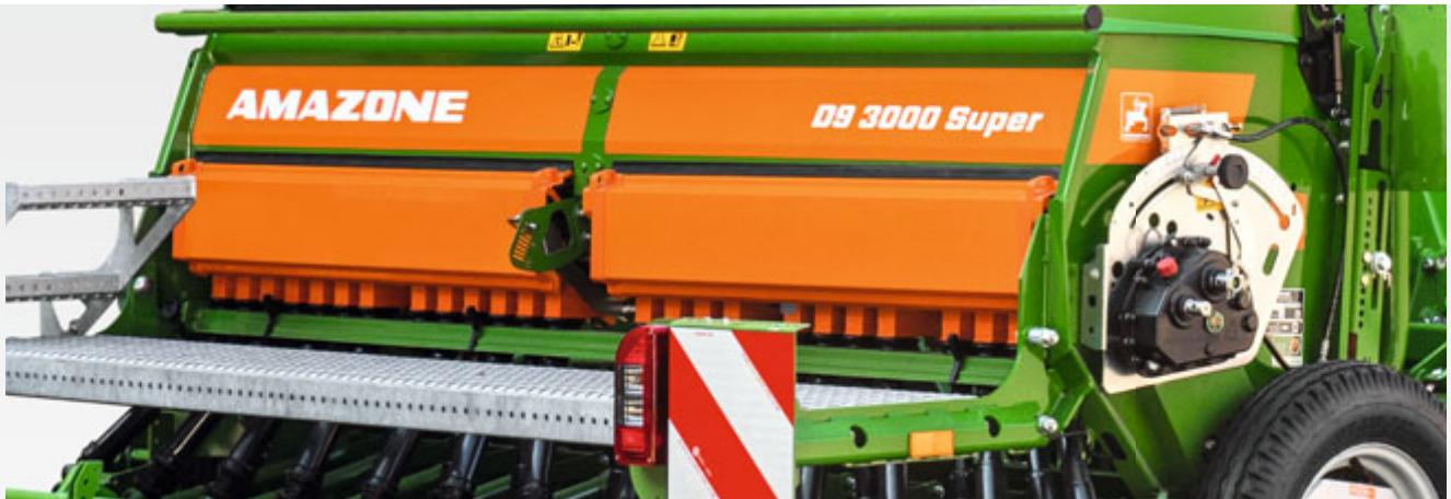
Seed hopper on the D9 with infinitely adjustable Vario gearbox
