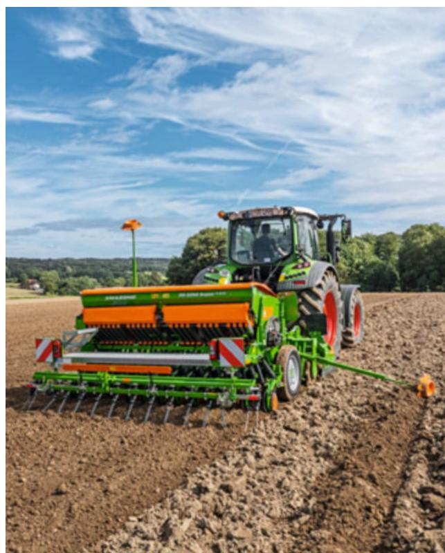
Simultaneous application of seed and fertiliser with the C-Drill fertiliser system saves on passes and can increase yields
