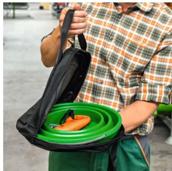
The standard calibration kit, with folding bucket and suspended weighing scales, is compact and practical to transport
