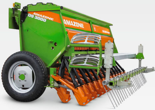
The D9 3000 mounted seed drill with WS suffolk coulters in solo operation
