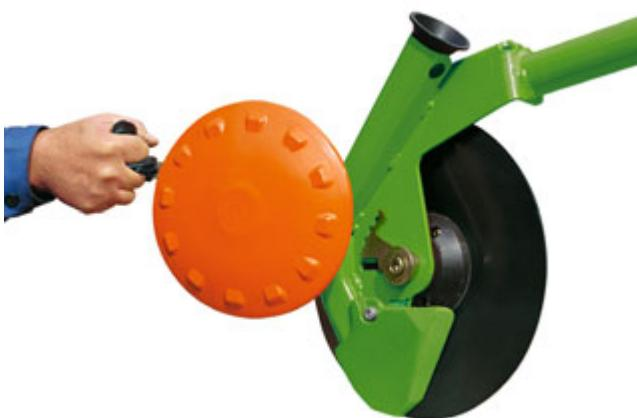
RoTeC coulter ( $\varnothing$  320 mm) with Control 10 depth guidance disc
