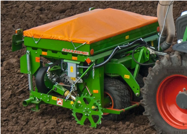
6 m Avant with twin-tip front tank and mechanical metering drive via a star wheel for two distributor heads
