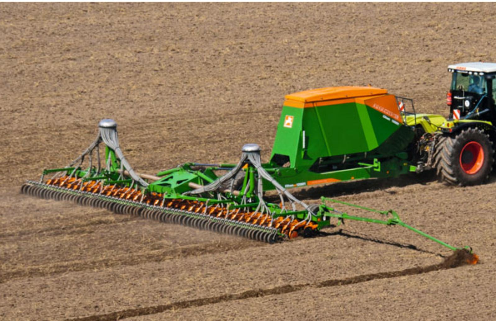
The Citan 12001-C and 15001-C offer the possibility to place, in addition to the seed, also fertiliser down in the seed furrow. For this reason, the hopper is divided and can be filled 2/3 with seed and 1/3 with fertiliser or a second kind of seed. If division of the tank is not necessary, it can be completely filled with one kind of seed. The metering is carried out via Vario gearboxes which can each meter seed rates of 2 to 400 kg per hectare.
