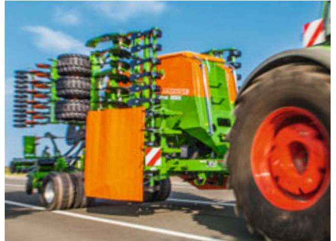
Both the Cirrus and also the Citan seed drills can be folded in to a transport width of 3 m in the shortest of time.
