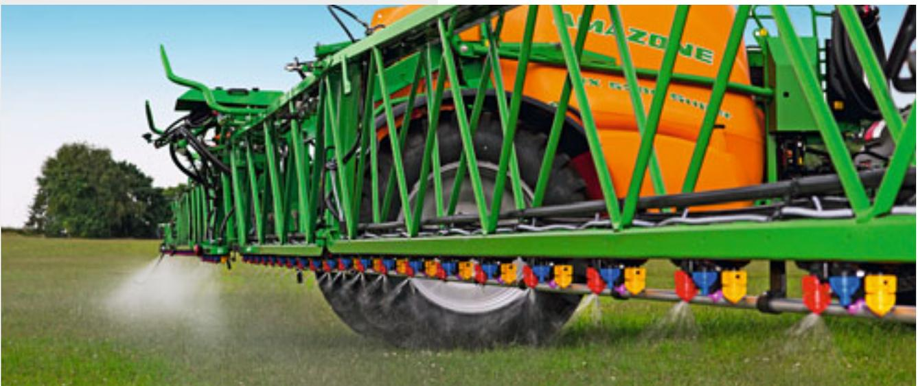
If AmaSelect and GPS-Switch are combined, part-width sections at a spacing of 50 cm can be controlled individually and this keeps the overlap zones down to a minimum. This is optimum, both from an economic and also an ecological point of view.
