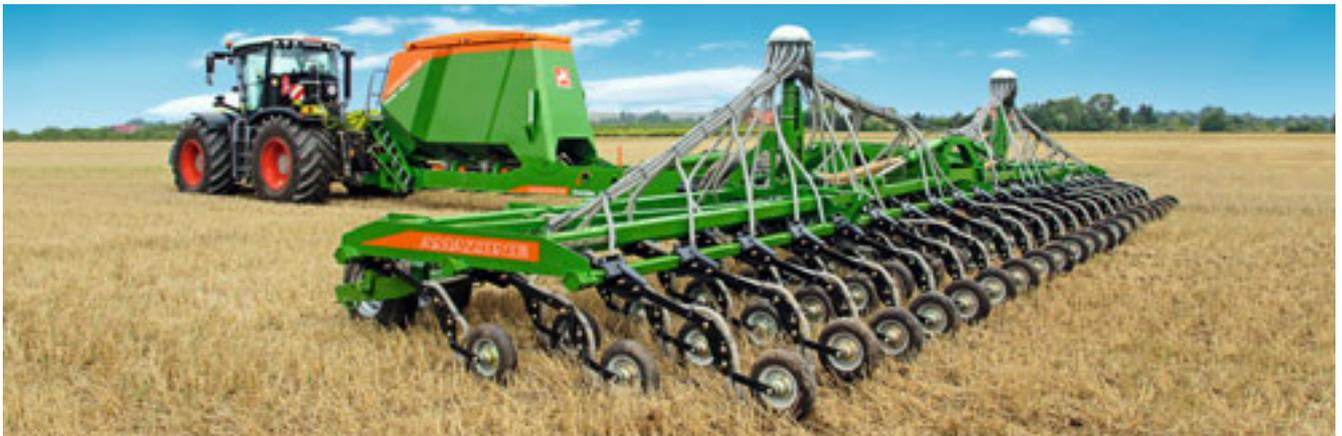
The Condor for direct sowing in dry soil conditions and large field sizes.
