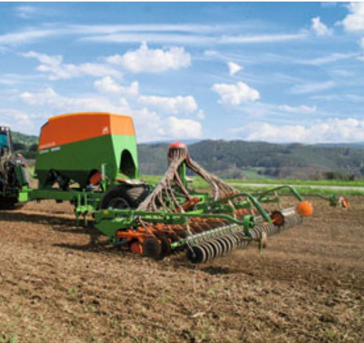
The Citan 6000, in a working width of 6 m, for operation with tractors from 120 HP.
