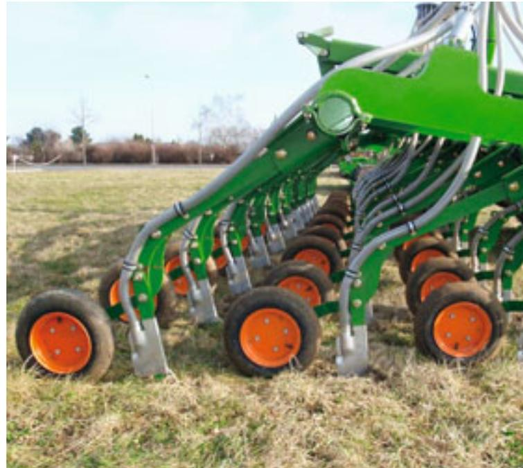
By means of the press wheel following the ConTeC coulters on the Condor, reconsolidation is achieved that ensures better seed-soil contact.
