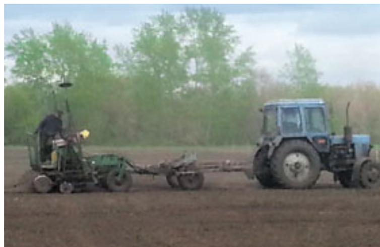
Method 2: Mechanical disc drill C3П in a 7.2 m working width on a Belarus MTS 50 (50 HP).
