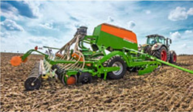
Cirrus is equipped with pre-cultivating disc elements and achieves daily outputs of 25 ha to 60 ha (depending on working widths of 3 m, 4 m or 6 m).
