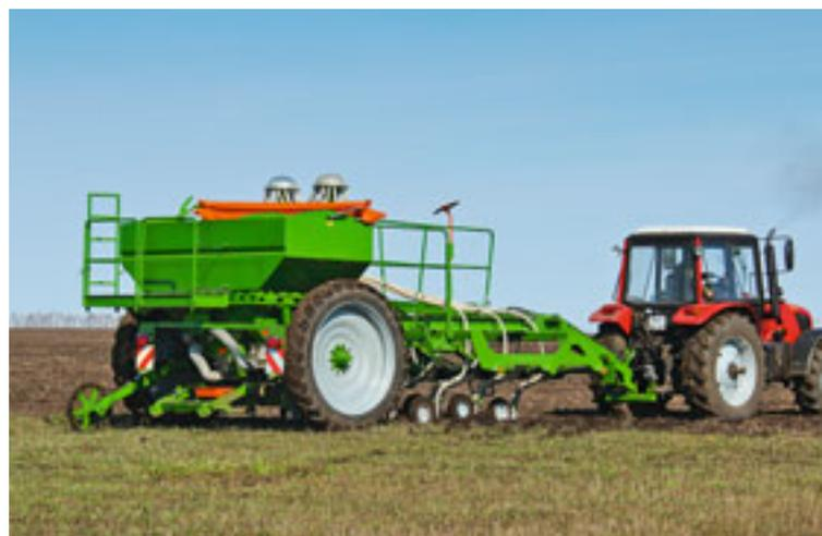
Method 1: Pneumatic seed drill 3 m with ConTeC coulters on a Belarus MTS 1221.4 (120 HP).
