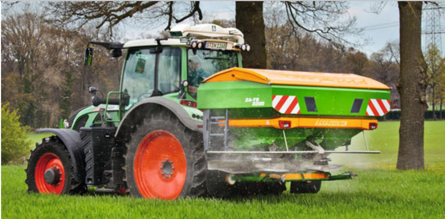
Fertiliser spreader and N-sensor for site-specific fertilisation.
