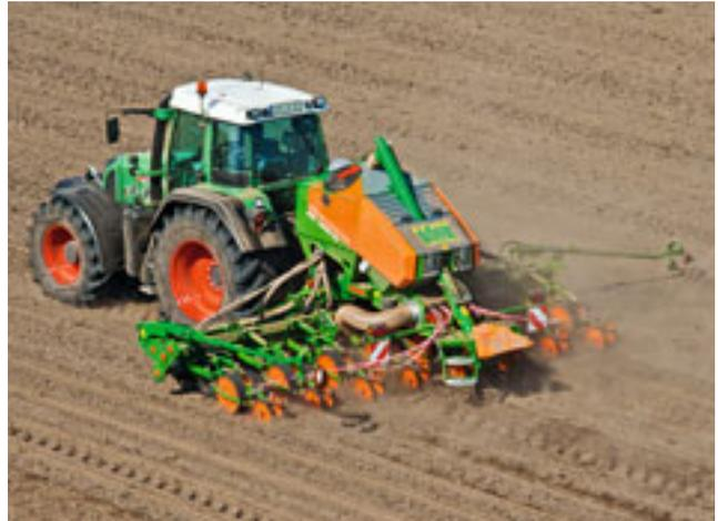
EDX 6000-2C with integrated fertiliser hopper, 8 rows and 6 m working width.
