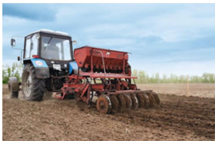
Method 3: C3C2.1 mechanical wing coulters seed drill with 2.1 m working width on a Belarus MTS 82.1 (80 HP).
