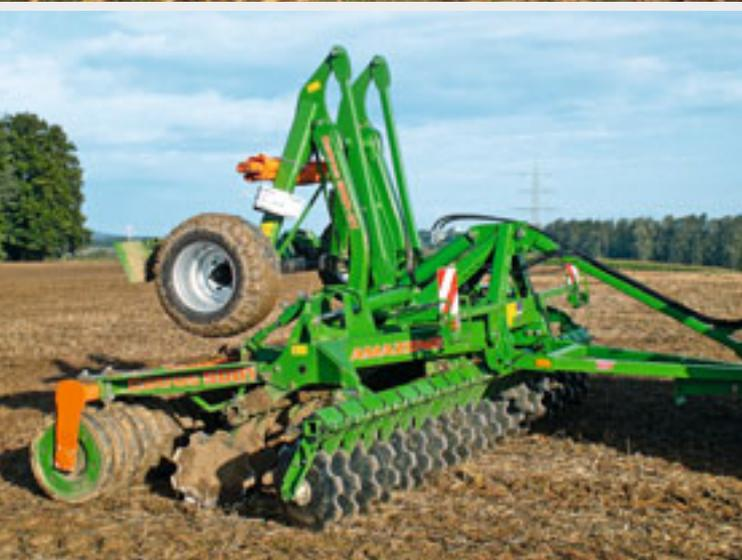
The standard equipment on the Catros-2 TS trailed machines in 4 m, 5 m and 6 m working widths includes a bogey chassis and drawbar.
