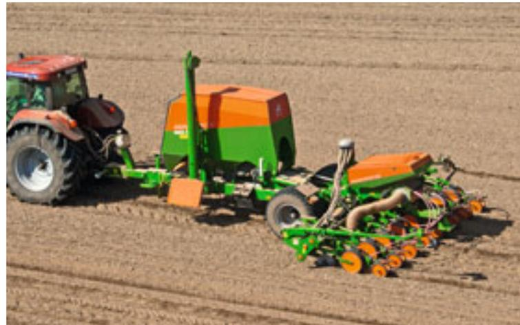
EDX 6000-T precision air seeder with 8 rows and 6 m working width.
