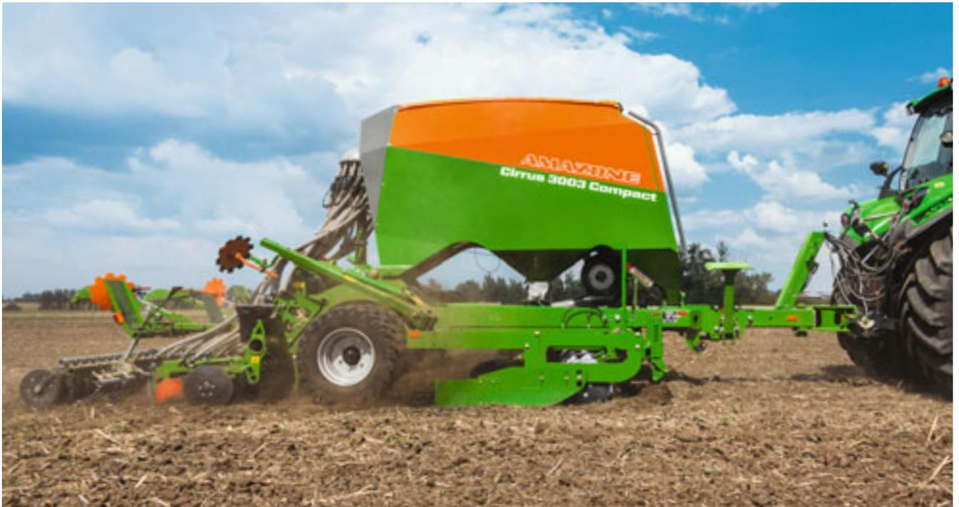
As a trailed sowing combination, the Cirrus makes higher operational speeds possible.
