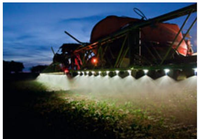
The work lights on the booms or LED individual nozzle illumination eases work after dark.
