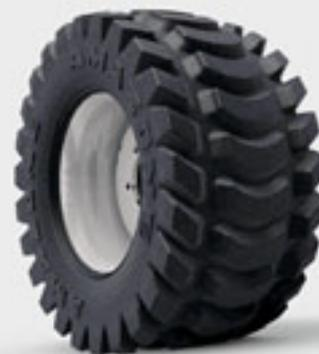
Thanks to the good wall flexing, the radial designed profile of the Matrix tyre virtually rests evenly on the soil across all the rows creating even germination conditions.
