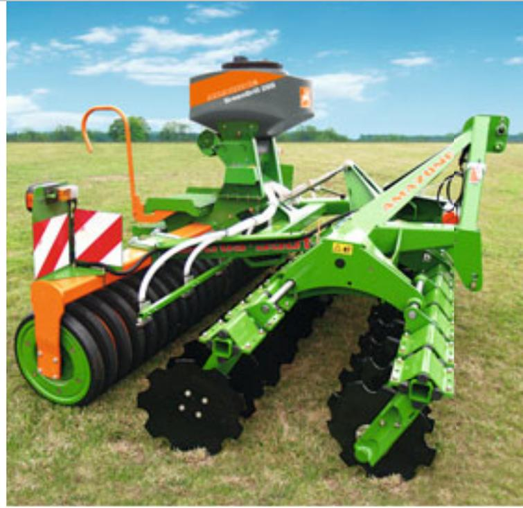
In combination with the GreenDrill seeder box, the Catros compact disc harrow can also be used for sowing fine seeds. Alternatively, the GreenDrill seeder box can also be operated with the Cenius mulch cultivator, the KG rotary cultivator or the KE rotary harrow.
