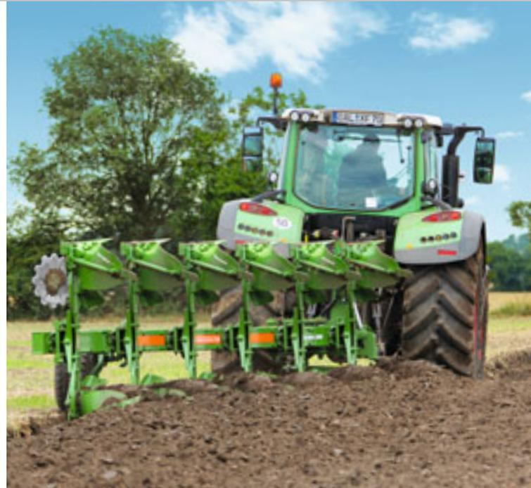
With its 83 cm frame height and smooth beam surface, the Cayron ensures especially good trash passage.
