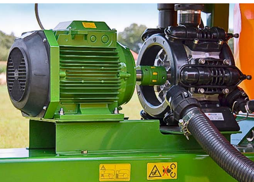
Electric pump drive
