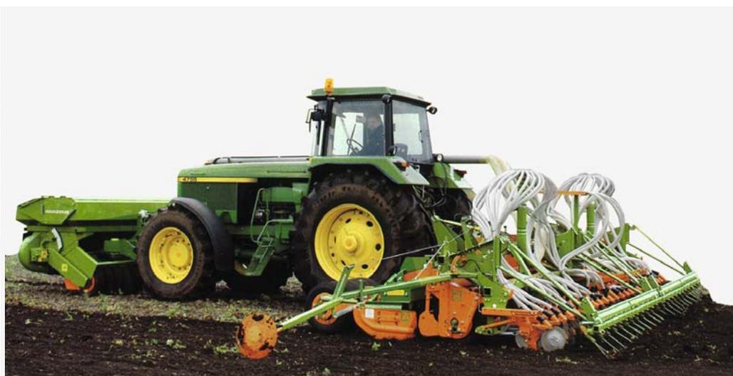
1995: Pneumatic front packer seed tank and 6 m rotary cultivator with tyre packer seed drill
