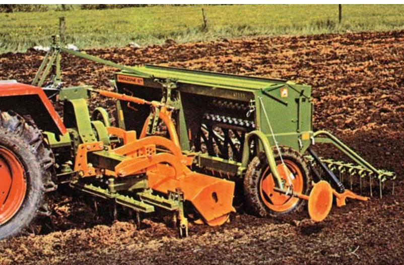
1972: D7 mounted seed drill with RE reciprocating power harrow, rigid tine bars and tooth packer roller
