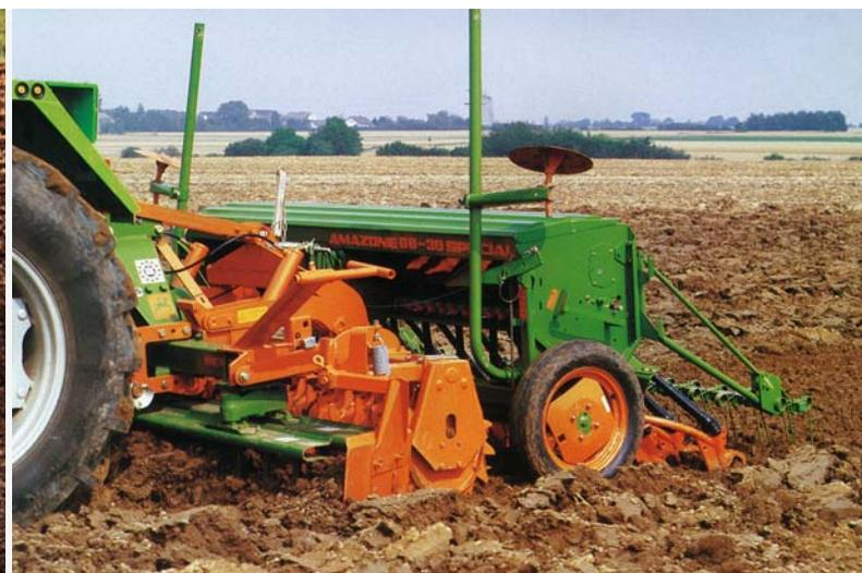
1985: D8-30 Special mounted seed drill with RE reciprocating power harrow and spring steel tine bars
