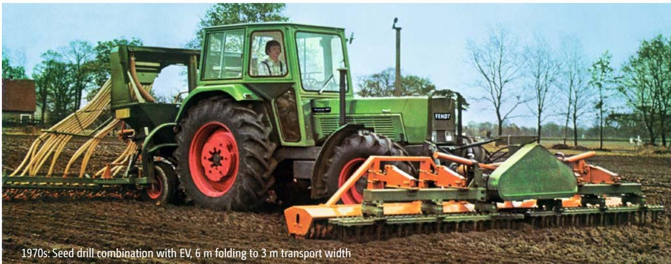
1970s: Seed drill combination with EV, 6 m folding to 3 m transport width
