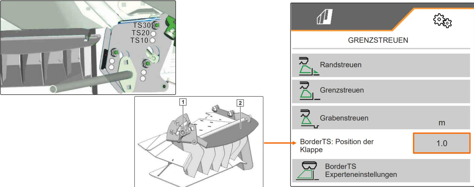
The diagram illustrates the setup for the BorderTS system. It shows the control panel with buttons for TS30, TS20, and TS10. A 3D model of the spreading vane unit is shown with callouts 1 and 2 indicating the flap position and the adjustment point. A screenshot of the machine's control interface shows the 'GRENZSTREUEN' menu with 'BorderTS: Position der Klappe' set to 1.0 m.
