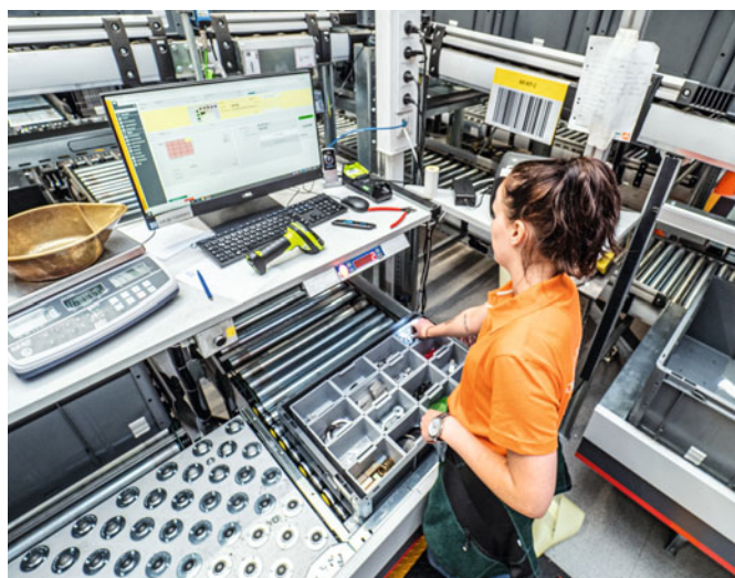
Workplace in the automatic small parts warehouse (ASPW)
