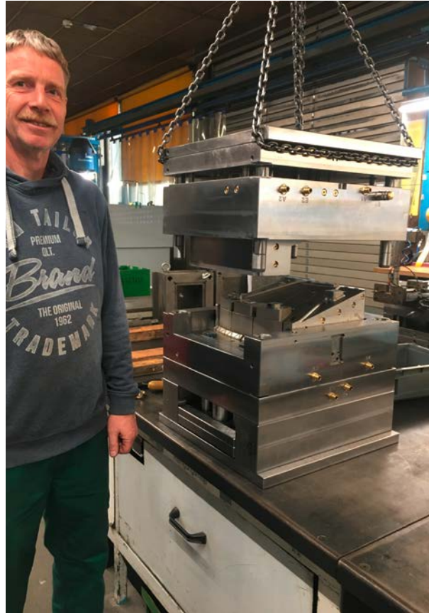
Plastic injection moulding tool from our own tool shop
