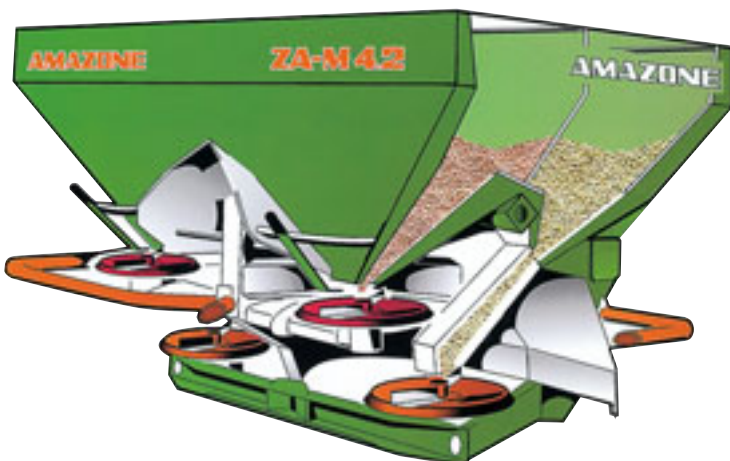
AMAZONE 'ZA-M 4.2': a fertiliser spreader which can spread two types of fertiliser at the same time, 1997
