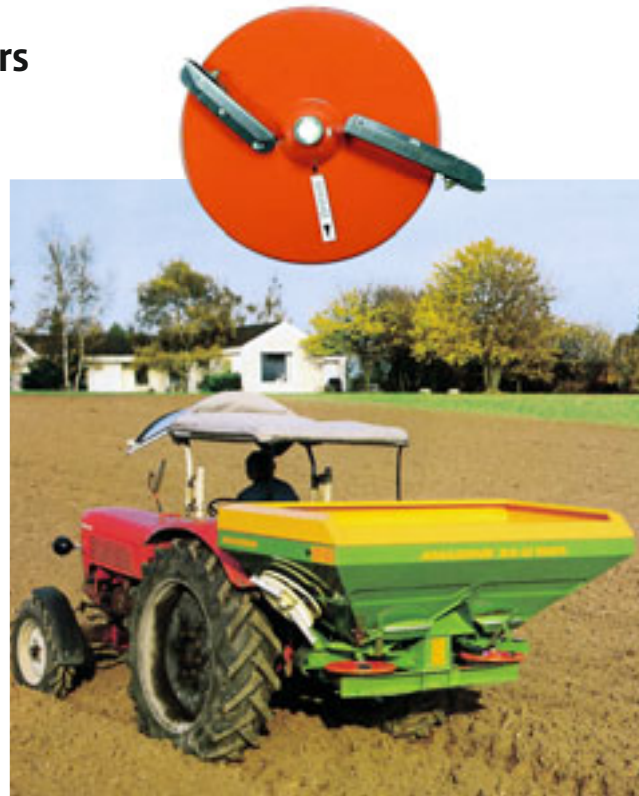
AMAZONE 'ZA-U' with tool-free interchangeable disc system
