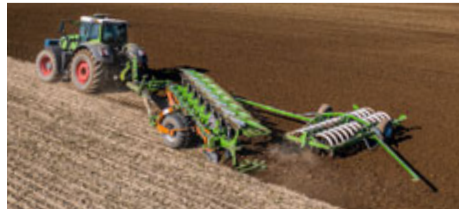
Above: Cobra 7000-2TX trailed shallow tine cultivator
