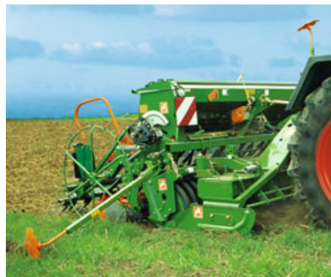
KG rotary cultivator with AD mounted seed drill in the field
