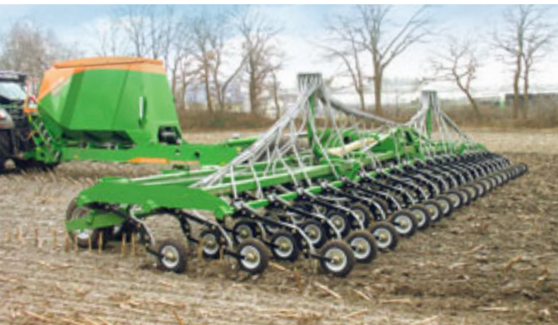
One of many innovations: the Condor tine coulter seed drill in up to 15 m working width
