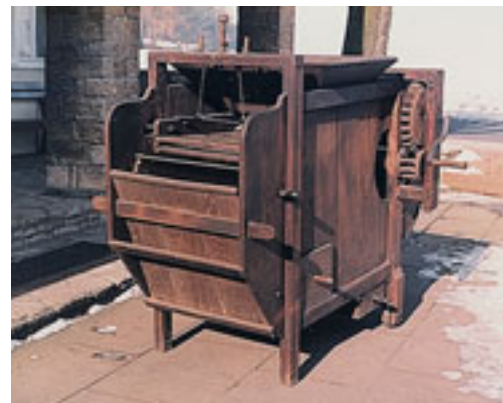
Dreyer's winnower from the 18th century, made entirely from solid oak wood
