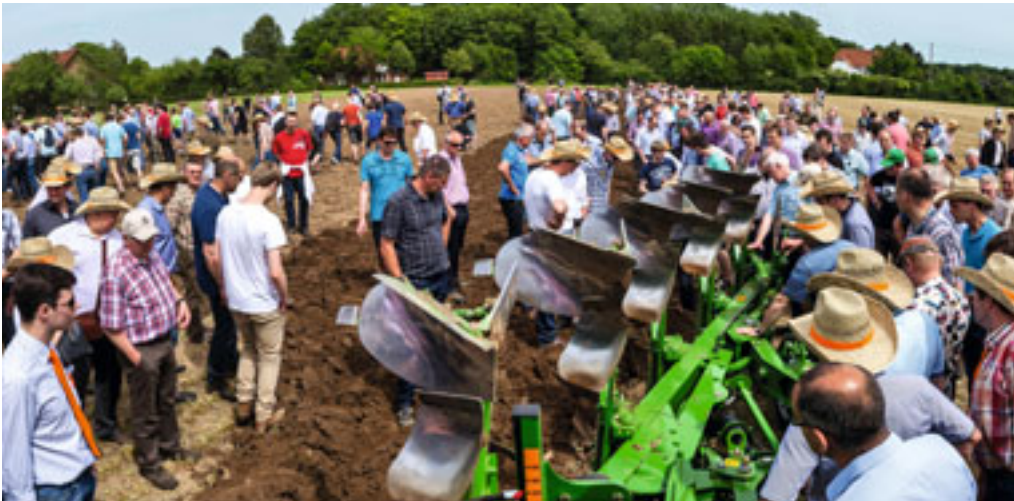
The new Cayron reversible plough in use at AMATECHNICA, 2014
