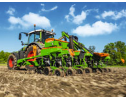
Precea 6000-2CC precision air seeder
