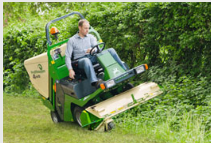
Right: Profihopper 4WDi with intelligent all-wheel drive, 2010
