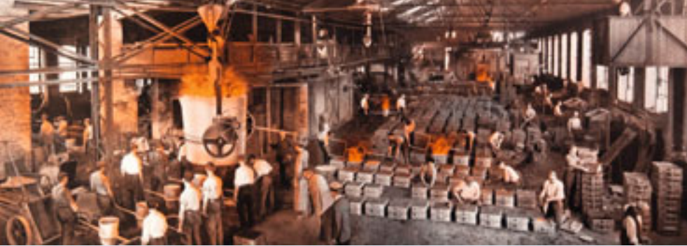
Steel foundry and tapping of the "Martin furnace" in the steel foundry
