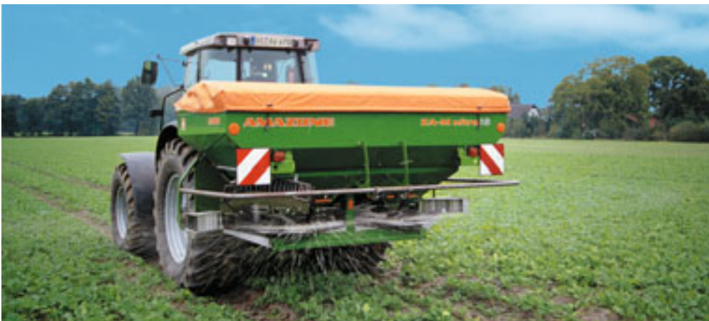
AMAZONE 'ZA-M ultra iS': the flagship of AMAZONEN- WERKE 2001 with 48 metre working width, GPS control and integrated weighing system
