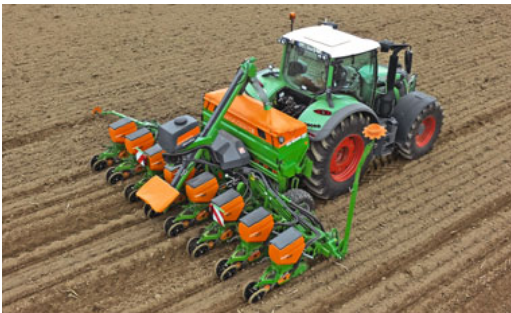
Precision air seeder 'ED 6000-2C', 2015
